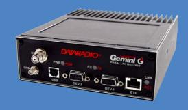
Capitalizing on over 20 years of experience designing mission critical wireless data equipment, Dataradio proudly presents the Gemini G3 700. This native IP mobile data modem operates at 128 kilobits per second in 50 KHz channels using proven FM technology.
